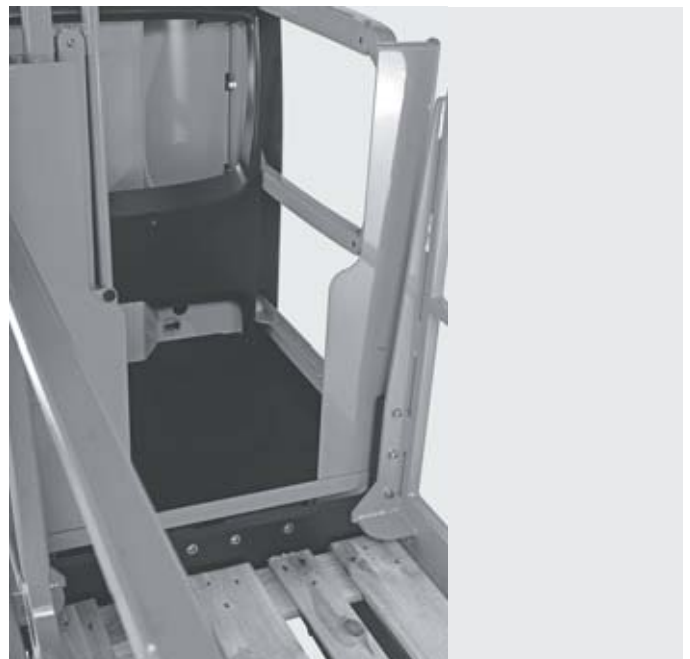
Easy and safe pallet access through open barrier
