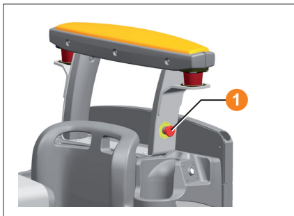
1 Additional emergency off switches (left and right-hand side of the truck)
